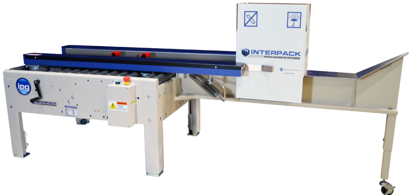
1 Self-tensioning & self-tracking drive belts simplify belt replacement
