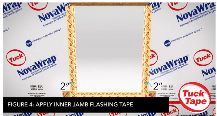
FIGURE 4: APPLY INNER JAMB FLASHING TAPE
